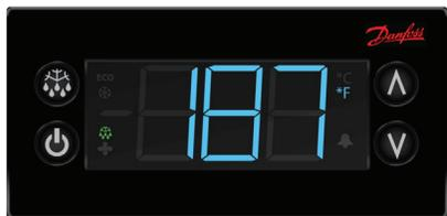
4. Scroll to **dis** using the up/down arrows and push the stand-by button (lower left button) to enter into the display menu.
