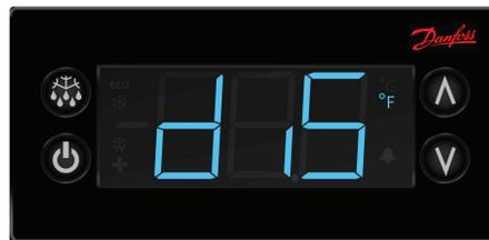
8. Push the defrost button (upper left button) to move out of the display menu and back to the normal display.
