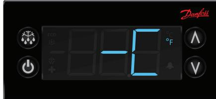
7. Push the defrost button (upper left button) to move out of the display unit menu.
