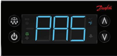
3. Scroll to **187** using the up/down arrows and push the stand-by button (lower left button) to enter.
