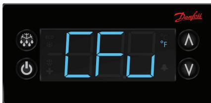
6. **-F** should be displayed indicating Fahrenheit. Use the down arrow to change it to **-C** for Celsius and hit the stand-by button (lower left button) to enter the change.
