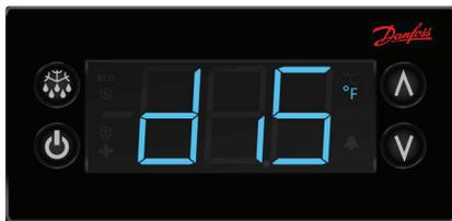
5. Scroll to **CFu** using the up/down arrows and push the stand-by button (lower left button) to enter the display unit menu.
