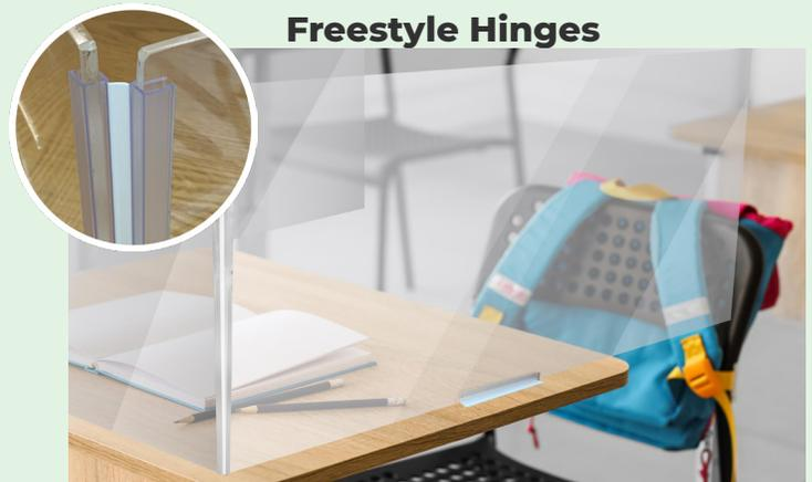
The "Freestyle Hinge" is an extruded PVC product and can flex when two panels are inserted and folded. Connects two acrylic or polycarbonate windows to create enclosures at 180° to 45° and fits 5mm or 6mm thick pieces.
