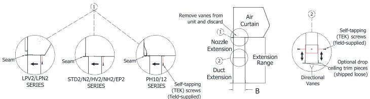
Note: Once unit and nozzle extension are installed, adjust duct extension to ensure the bottom is about 1" above door header
