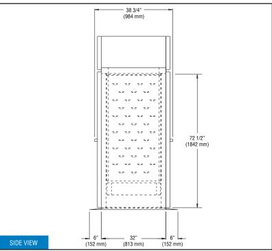
**IMPORTANT NOTE:** If the cabinet is located directly against a wall and/or under a low ceiling, a <u>minimum</u> clearance of 12" is required on top and 3" on sides.
