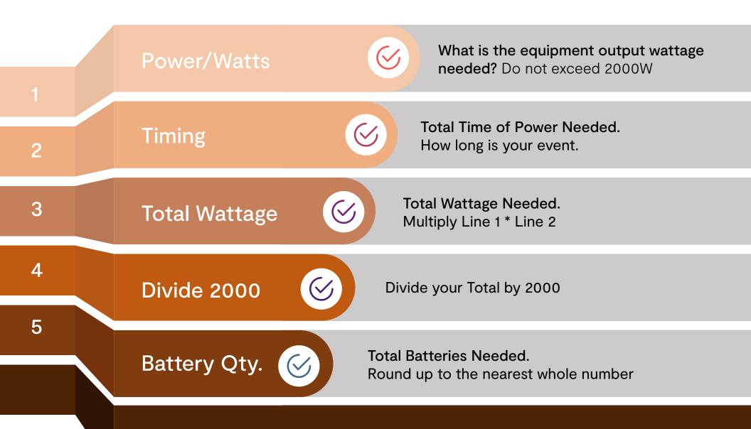
To determine the amount of main batteries divide #1 - power watts by 2000
