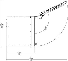
Max clearance required for opened door is 49-3/4" when opened to 90°\* (dimensions shown are without door overlay installed.)
