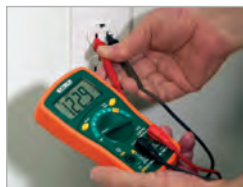
Displays AC Voltage of an outlet receptacle
