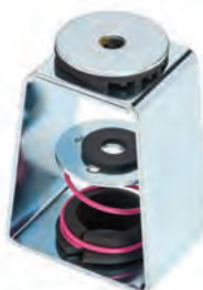
CH30SCS Type Deflection Combination Hanger 15° Tilt Spring & Neoprene w/ Seismic Cushion Stop 1" & 2" Deflection Pages 70 & 71
