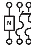
Fusible, Two-pole, 120/240 and 240 Volts AC; 250 Volts DC; Three-wire solid neutral, 240 Volts AC
