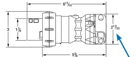
VersaMate® clamps provide a firm fit for one plug (or connector) over a wide range of cable diameters (competitors often need two - requiring additional sizing decisions).
