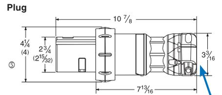
VersaMate® clamps provide a firm fit for one plug (or connector) over a wide range of cable diameters (competitors often need two - requiring additional sizing decisions).
