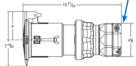
① Components are intermateable & UL classified with Appleton® Powertite® or Crouse-Hinds® Arkrite® devices (when installed in accordance with instructions furnished with device. Assemblies containing components from other manufacturers would have the NEMA type rating of the lowest rated device.
