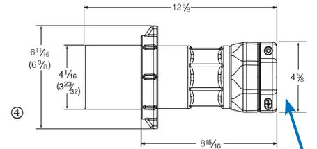
VersaMate® clamps provide a firm fit for one plug (or connector) over a wide range of cable diameters (competitors often need two – requiring additional sizing decisions).
