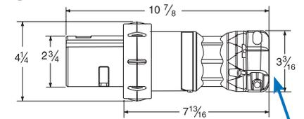
VersaMate® clamps provide a firm fit for one plug (or connector) over a wide range of cable diameters (competitors often need two – requiring additional sizing decisions).
