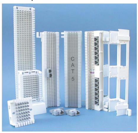
Hubbell Premise Wiring offers industry standard modular 66 blocks to add to its family of cross connect products. These blocks are used in equipment rooms and intermediate telecommunication closets to connect voice and data network wiring to customer premises equipment. Additionally, 66 blocks are used to expand Legacy systems or as a cost-effective, high-density, small scale cross connect for voice applications.
