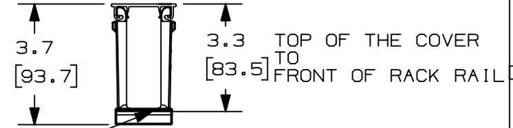
SURFACE IN CONTACT WITH FRONT OF THE RACK RAIL
