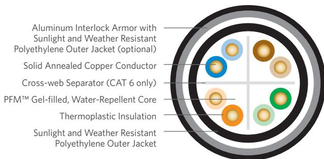
Aluminum Interlock Armor with Sunlight and Weather Resistant Polyethylene Outer Jacket (optional)
