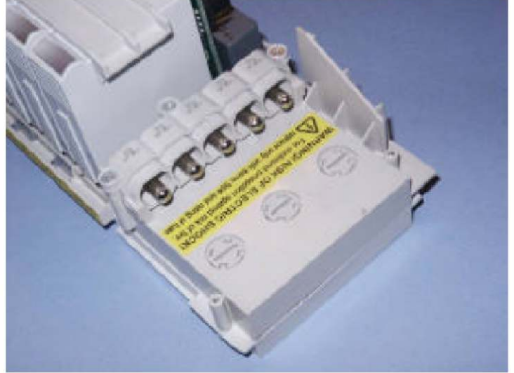
Step 3: Use a large flat blade screwdriver to turn the appropriate fuse ejector a quarter turn (90 degrees).
