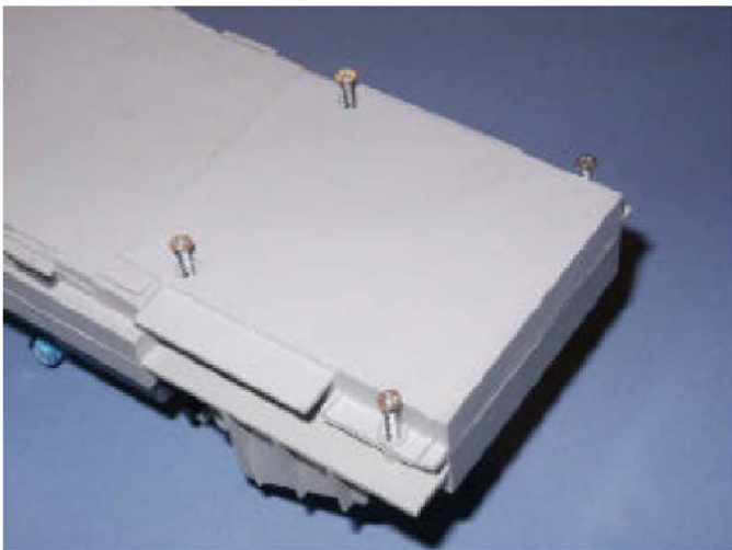
Step 2: Turn over, and remove the four screws holding the fuse cover in place. These screws are tight – use correct screwdriver size to avoid damaging screw head.
