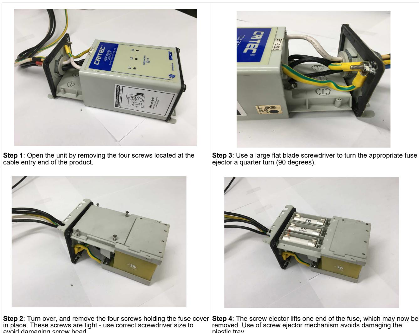
**Step 1:** Open the unit by removing the four screws located at the cable entry end of the product.
