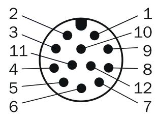
M12, 12-pin male connector, A-coded
