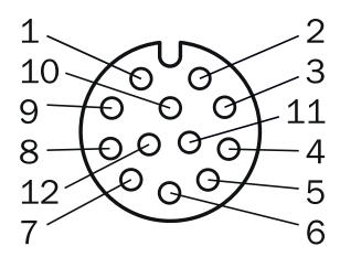
M12, 12-pin female connector, A-coded (I/O)
