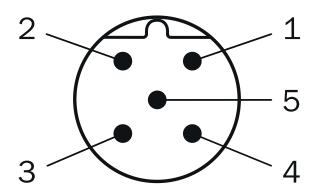
Male connector M12, 5-pin, A-coded
