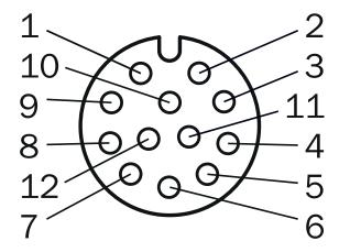
M12, 12-pin female connector, A-coded
