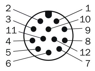
M12, 12-pin male connector, A-coded
