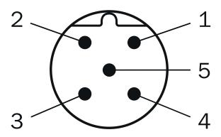
Male connector M12, 5-pin, A-coded
