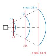
The specified numerical values are typical values and apply in the central 80% of the detection area, at room temperature, without ambient light, and at a frame rate of 25 fps. At distances > 9 m, the reliability of the measured values will be lower and individual pixels or pixel groups may exhibit faulty measured values. The measurement accuracy may degrade by up to  $\pm$  10 mm (typically  $\pm$  5 mm) over the entire ambient operating temperature.
